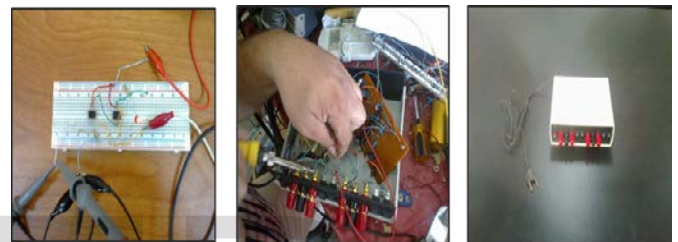
Fig. 3 Couple of digital images for the assembly process of the proposed amplifier: (a) initial design laid on electronic pinboard for testing, (b) internal view of amplifier, and (c) stand-alone final product (amplifier)
